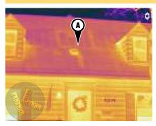
The solution to just about any problem involves first understanding the underlying causes. Ice dams are the result of a complex interaction of many things including architecture, climate and lifestyle. To put a finer point on it, ice dams are related to how heat escapes from the areas it belongs to areas it is not supposed to be. That heat causes snow melt on your roof, and the saga begins.
