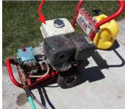
Busted. This local company uses a low-volume 4000psi pump to wash cedar roofs.
