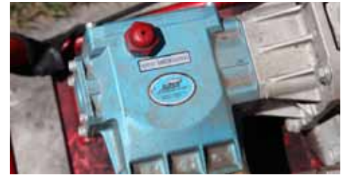
Busted. This local company uses a low-volume 4000psi pump to wash cedar roofs.
